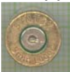
9 mm Luger, 3055 bar, 44300 psi Zündhütchen flach, schmale Ringfuge
