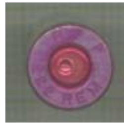
.222 Rem , 4810 bar, 70000 psi No signs of high pressure
